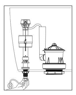
With correct washers in place (see Step 9a), tighten COUPLING NUT 1/4 turn beyond hand tight.
